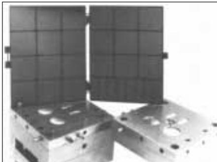
NTMA Surface Finish Reference Guide Sheet is included with each book. Detailed are 29 different surfaces produced by various finishing processes. The sheet finishes are keyed by number to matching numbers molded into the specimen book. Sheet finishes below are also represented in Superior's FORTAL Mold Cavity Specimen Book.
