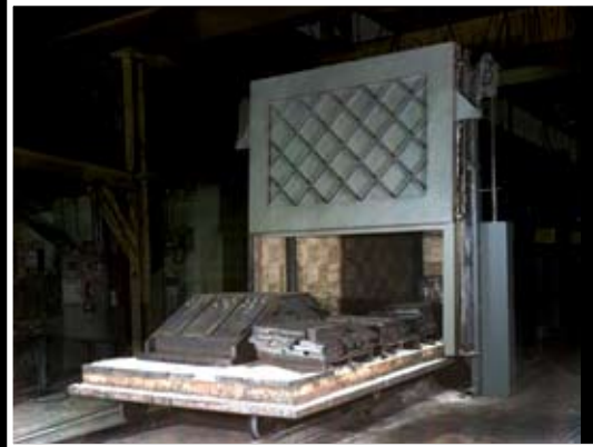
Stress Relieving: Assures uniform material characteristics.
