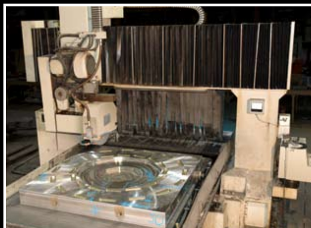
Large Capacity Surface Grinding: "Bridge type" flat and parallel finishing for all plate thickness. High micro-finishing down to 32 micro.
