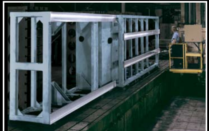
Large Fabrication Horizontal Milling Capacities: Plate and weldment assemblies to 50 feet are finished machined by Superior's in-house machining equipment.
