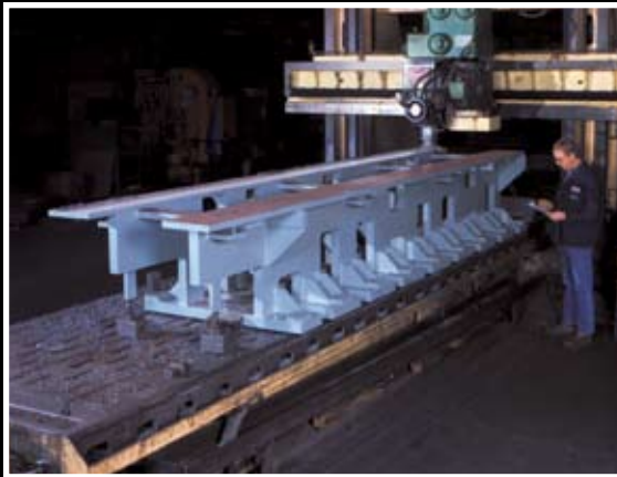
Large Capacity Milling: Long and narrow plate and fabricated assemblies are easily surface milled for flatness and parallelism.
